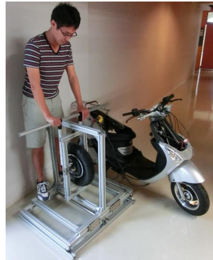
Fig.7 Experimental apparatus by using in-wheel motor
