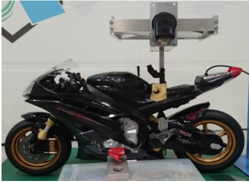
Fig.2 RC toy bike with gyro actuator
