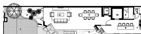
1ST STOREY PLAN 1 LAMP 6 BATHROOM 2 WATER FEATURE 7 MASTER BEDROOM 3 LOBBY 8 METAL ROOF 4 DINING 9 BAZILLAH 5 KITCHEN 10 BAZILLAH WITH GREEN WALL 11 LIFT
