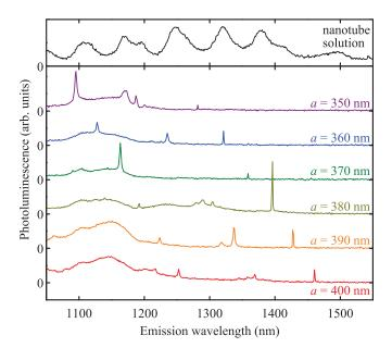
FIG. 3. The top panel shows a PL spectrum from nanotube solution taken with an excitation wavelength of 774 nm. The bottom panel shows PL spectra for devices with  $r = 100 \, \mathrm{nm}$  and a ranging from 350 nm to 400 nm, taken with an excitation wavelength of 750 nm and a power of 0.5 mW. The curves are offset for clarity.
