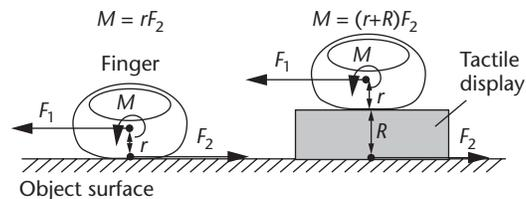
**3 Effect of system thickness. The contact generates frictional force, which the finger perceives as a torsional moment. If the distance between object surface and display surface increases, it generates greater torsional moment, creating an unnatural haptic sensation.**
