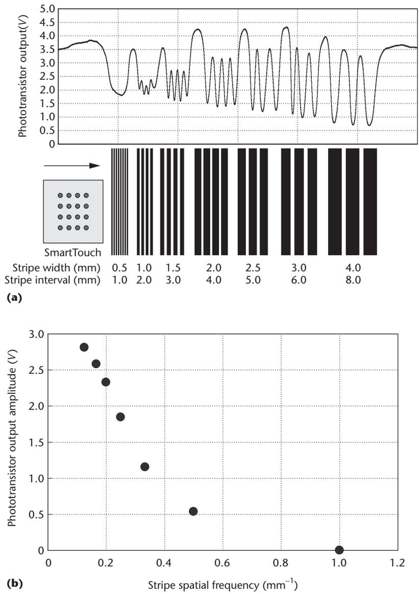
object. Because we didn't embed a light source into the system, an LED lamp lit the paper from below.
