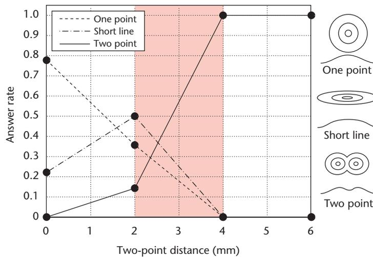
**9 Two-point discrimination with anodic pulse stimulation. The static resolution is 2 to 4 mm.**
