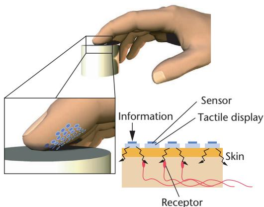
**1 Augmented reality of skin sensations. A new functional layer of skin composed of a sensor and display acquire and convert surface information about an object into tactile information for display.**
