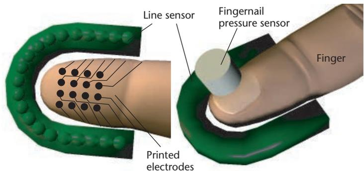
By changing the sensor, other modalities of sensation can be translated to touch as well. We are now considering the combination of a tactile sensor matrix with an electro-tactile display to perform tactile-to-tactile conversion. If the tactile sensor is more sensitive than human perception (the detection threshold of skin surface deformation is about  $0.01 \text{ mm}^{10}$ ), we can enhance the natural tactile experience.
