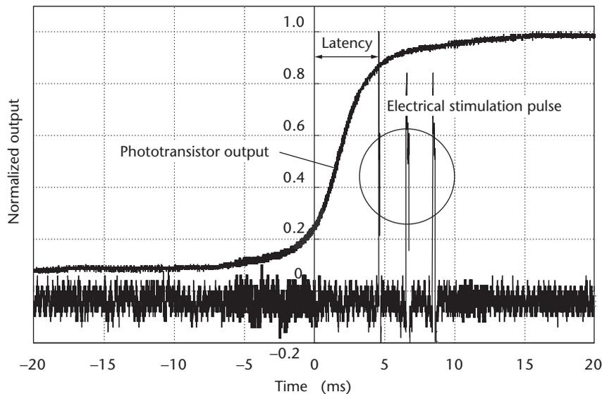
**5 Phototransistor output and stimulus current (normalized). The latency between sensing and stimulation was less than 4 ms.**
