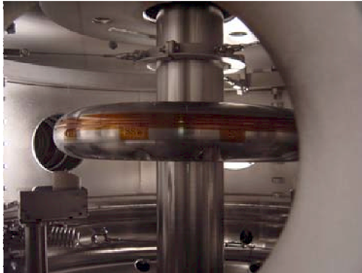
Figure 2.4: Picture of the levitated internal coil
