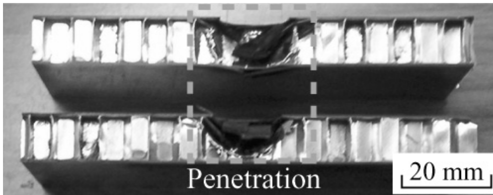
Fig. 2.8 Photograph of impacted specimen with UM55 facesheet.
